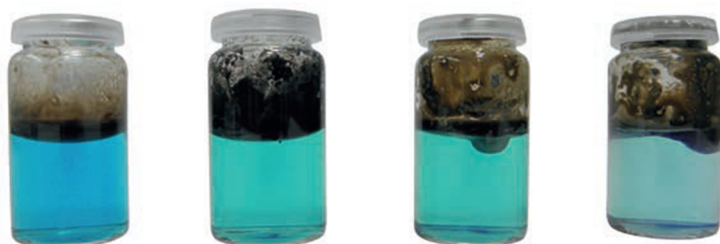
Examples of Different Total Iron Concentration Measured in cylinder drain oil (CDO) Samples
